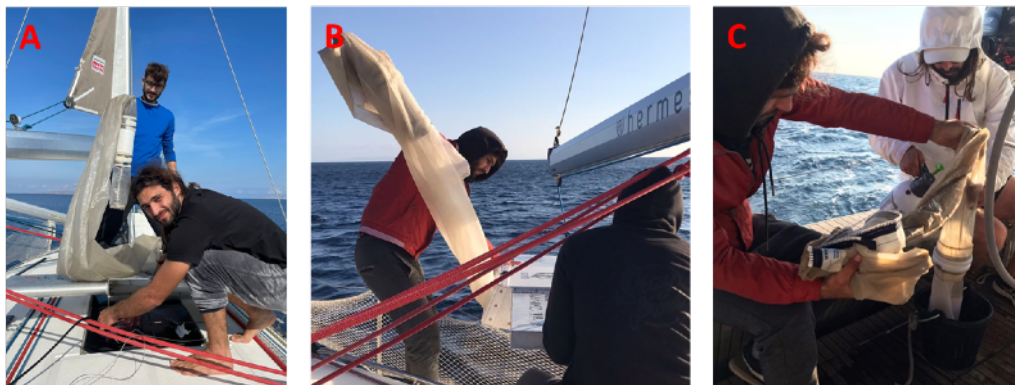
Figure 1: Preparing the manta trawl (A), taking the trawl out of water after sampling (B) and washing the net for sample collection in a sieve (C).
