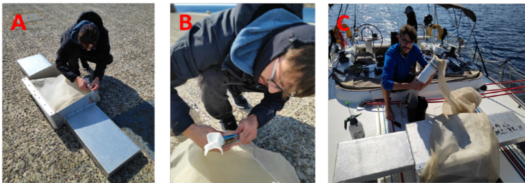
Figure 1: Assembling the Manta Trawl (A) and the flowmeter (B) on land and preparing the net for sampling on board (C).
